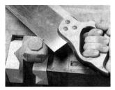
**Fig.7** Undercut the corners to remove the waste.
