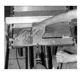
**Fig.16** Drilling the Sockets in the Drawer Front ends.
