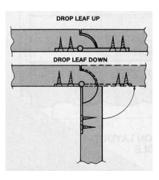
**Fig.20** Hinge pin-to-rule joint relationship
